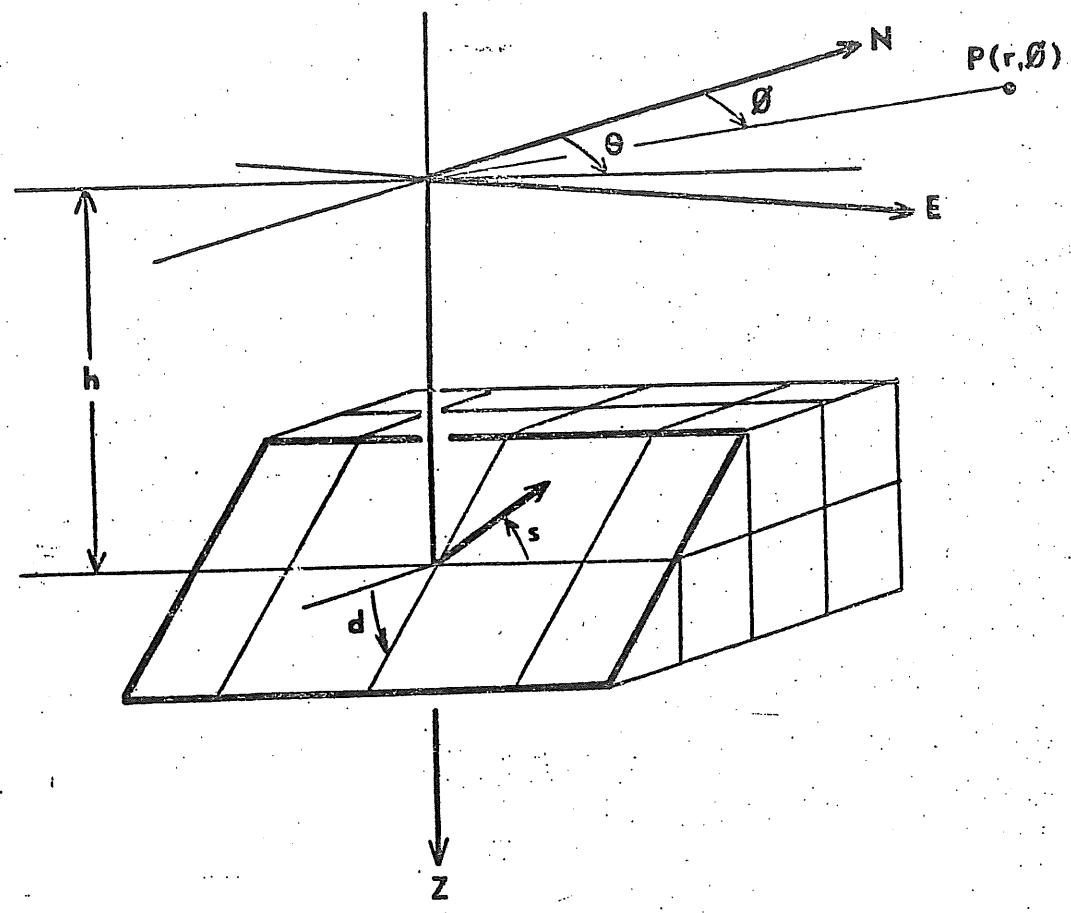
Fig. A.1. Coordinate and fault plane geometry
