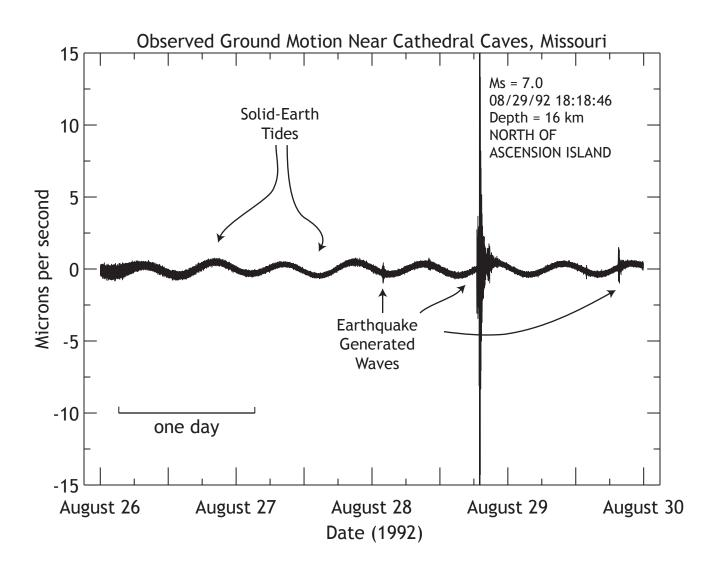
The Earth constantly vibrates as a result of the tidal forces between the Sun, Moon, and Earth, as well as atmospheric and ocean interaction with the ground. The above seismogram shows the velocity of the ground in central Missouri, U.S. resulting from atmospheric, tidal, and several earthquake, the largest vibrations were generated by a magnitude 7.0 earthquake near the Mid-Atlantic Ridge, off the west coast of Africa.
