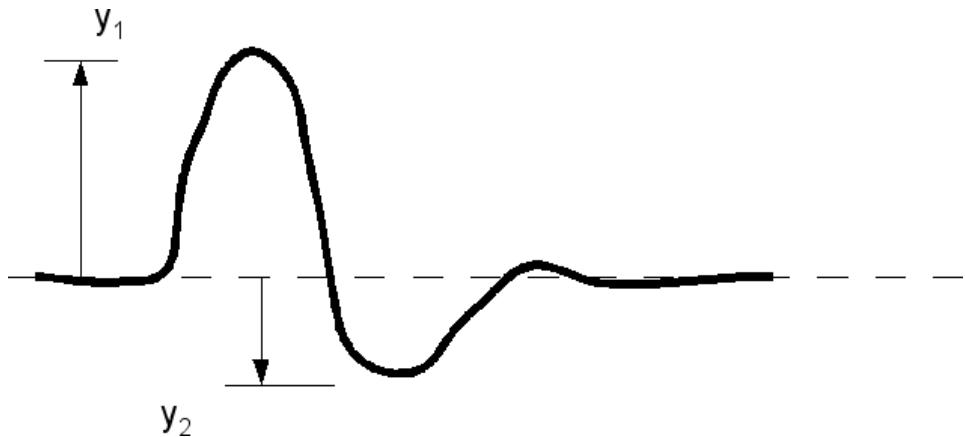
Call the first throw  $y_1$  and the second, much smaller one,  $y_2$ . If there were no friction,  $y_1/y_2$  would give us the damping ratio  $\varepsilon$ . But the effect of friction is equivalently to shift the zero line upward during the stroke from the turning point of  $y_1$  to that of  $y_2$  by a distance  $r$  the method of finding which we shall next describe. Hence we correct our observation by subtracting  $r$  from  $y_1$  and adding it to  $y_2$ . The formula will therefore be
