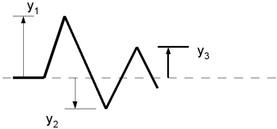
The effect of linear friction is to subtract a constant amount from the amplitude of successive swings. Let the decrease in amplitude for each quarter swing be  $r$ . Then, since there are four quarter swings between the turning point of  $y_1$  and that of  $y_3$ , the difference  $y_1 - y_3$  will be  $4r$ . Hence we have the formula
