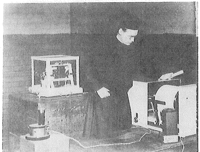
Reverend John P. Delaney, S. J. with the Galitzin-Wilip vertical component seismograph
