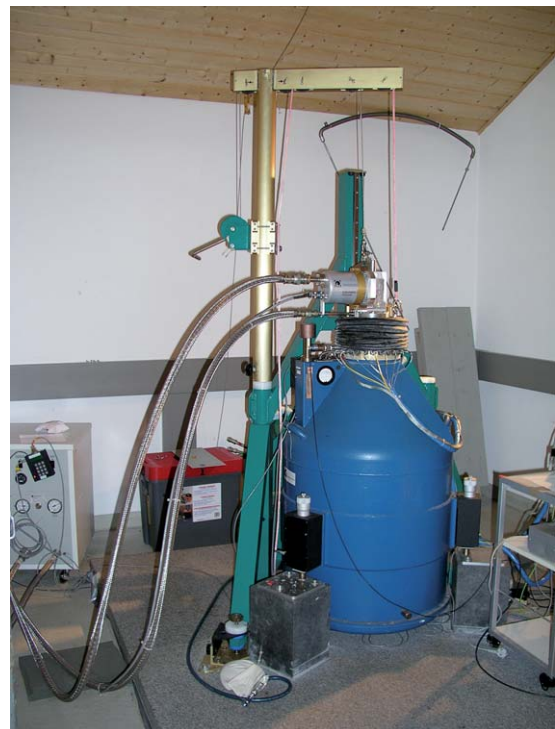
Figure 5 One of the first dual-sphere instruments (CD029, now at Wettzell, Germany) with a ULHD using a Leybold KelKool 4.2 K GM coldhead. The support cranes used to insert and remove the coldhead are shown in the background.
