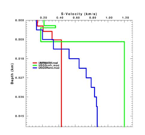
This effort investigates the feasibility of inverting Pwave first arrivals and Rayleigh-wave phase velocities obtained using a vertical hammer source and vertical geophones and SH-wave first arrivals and Love-wave dispersion obtained using horizontal hammer sourced and horizontal geophones.
