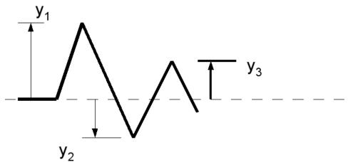
The effect of linear friction is to subtract a constant amount from the amplitude of successive swings. Let the decrease in amplitude for each quarter swing be r. Then, since there are four quarter swings between the turning point of  $y_1$  and that of  $y_3$ , the difference  $y_1 - y_3$  will be 4r. Hence we have the formula
