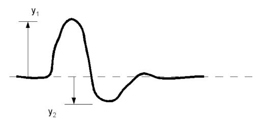
Call the first throw  $y_1$  and the second, much smaller one,  $y_2$ . If there were no friction,  $y_1/y_2$  would give us the damping ratio  $\varepsilon$ . But the effect of friction is equivalently to shift the zero line upward during the stroke from the turning point of  $y_1$  to that of  $y_2$  by a distance *r* the method of finding which we shall next describe. Hence we correct our observation by subtracting *r* from  $y_1$  and adding it to  $y_2$ . The formula will therefore be
