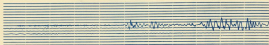
Figure 2—Portion of the Sprengnether series A. B. seismogram for 29 September 1930 recorded at St. Louis, Mo. Illustrates body and surface waves for an earthquake off the Pacific coast of Mexico near 28° north latitude, 101° west longitude, origin time 05:05:15.5 Greenwich. The S-P distance for this record by Chart II is 1760 miles.
