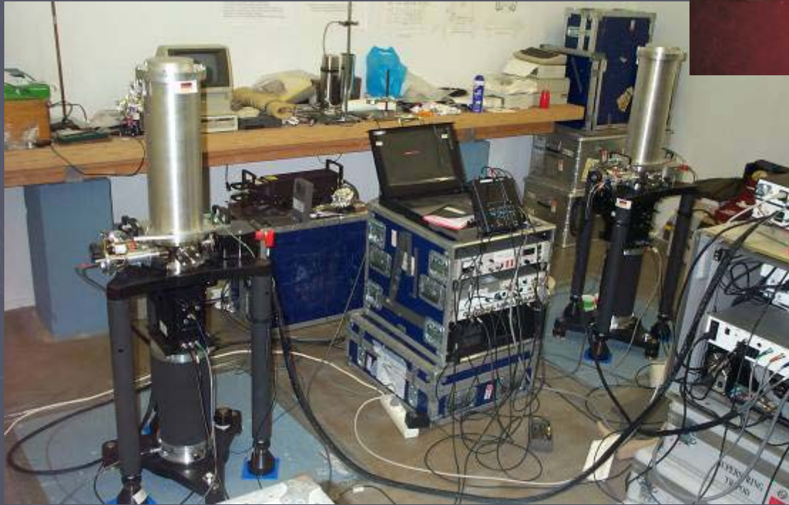
Fig. 7 Parallel measurements with FG5-220 (IfE) and FG5-221 (FGI) at station Metsähovi in Finland.
