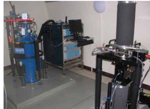
Figure 4. GWR model SGT48 operating in Hsinchu, Taiwan. The dewar sits on the ground, and can maintain liquid helium indefinitely. Shown with a standard electronics and data acquisition package, and also an AG.
