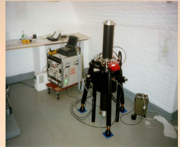
FG5#206 Absolute gravimeter (calibration, long term drift of SG)
