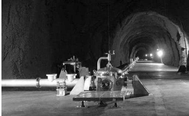
Figure 9. View of the 100m laser strainmeter system in the Kamioka mine, Gifu, Japan.
