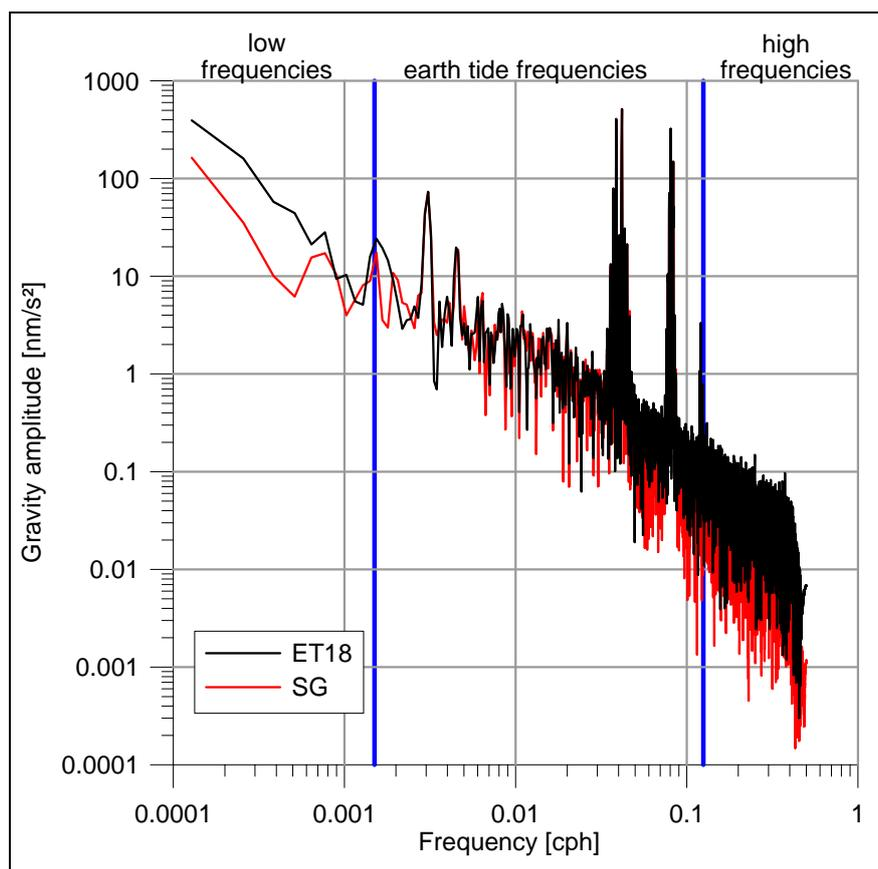
**Fig. 2:** Spectra of the ET18 gravimeter and the SG gravimeter over the whole frequency range.
