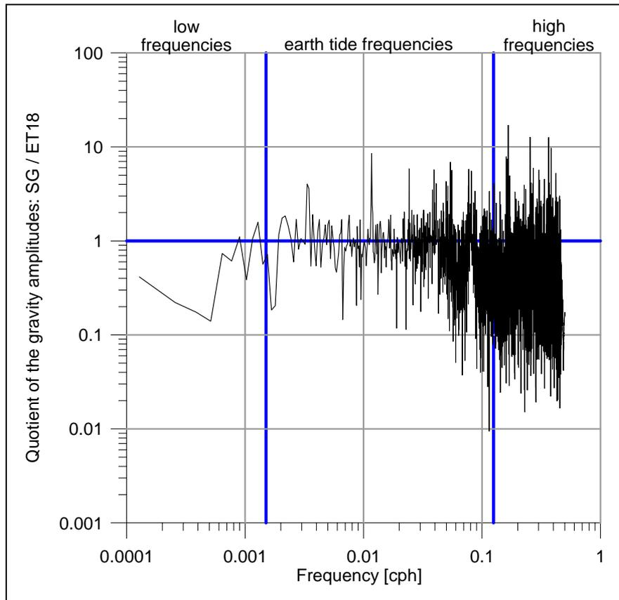
**Fig. 3:** Transfer function between the ET18 gravimeter and the SG gravimeter over the whole frequency range.
