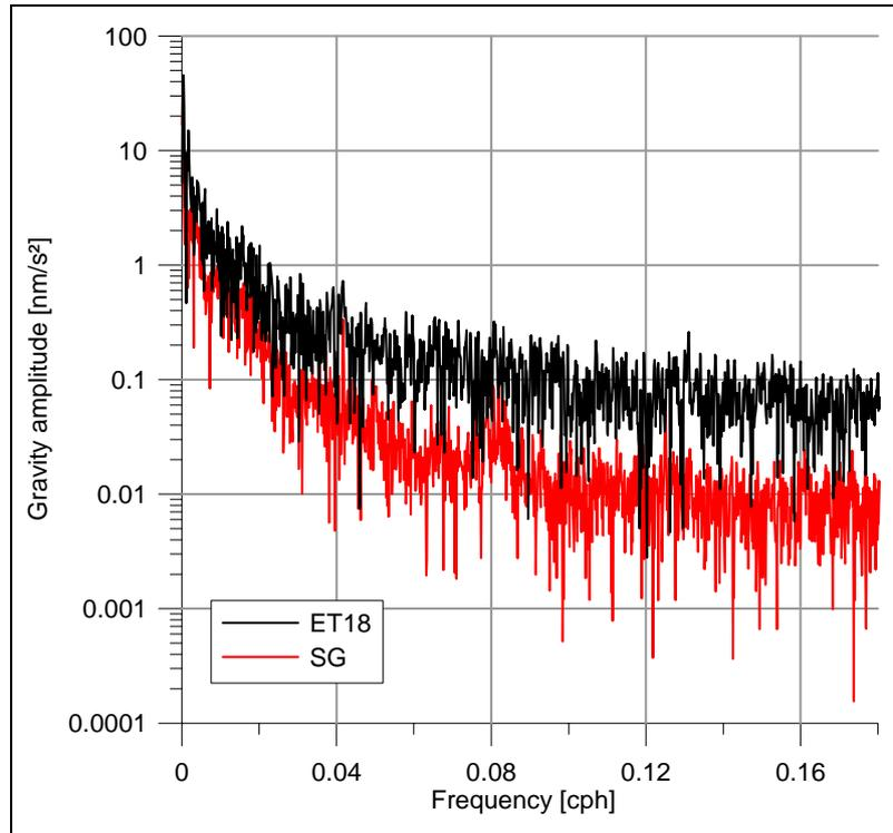
**Fig. 5:** Frequency spectra of the residuals from tidal analyses for the ET18 gravimeter and SG gravimeter.
