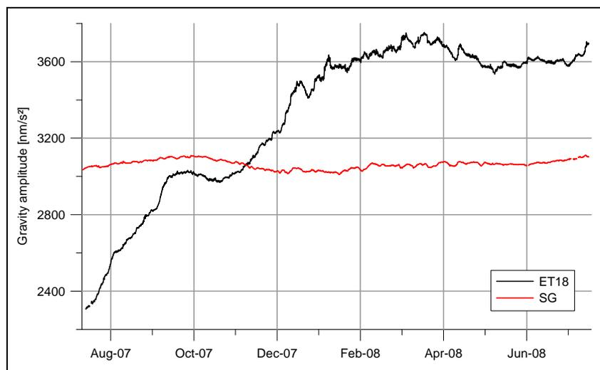
**Fig. 4:** Long-term drift of the ET18 gravimeter and the SG gravimeter. Both records contain waves with periods longer than 28 days.
