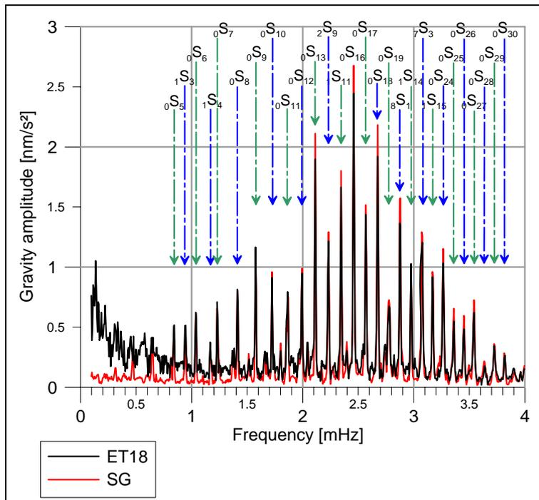
Fig. 7: Stacked spectra of three earthquakes of the ET18 and the SG gravimeter with 28 spheroidal free modes of the Earth.
