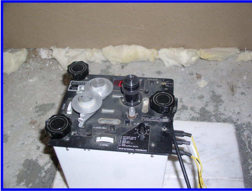
Figure 1: Gravimeter D-218 in the measuring room of Aswan station.
