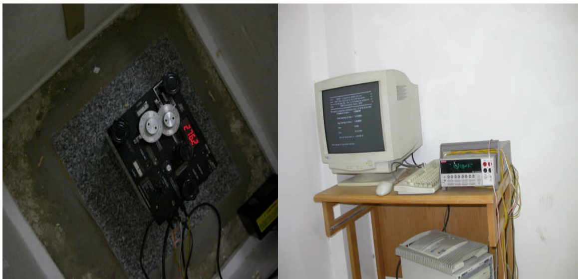
Figure 3. Lacoste and Romberg Gravimeter D-218 in the measuring room of Hurghada station (left) and recording system (right).
