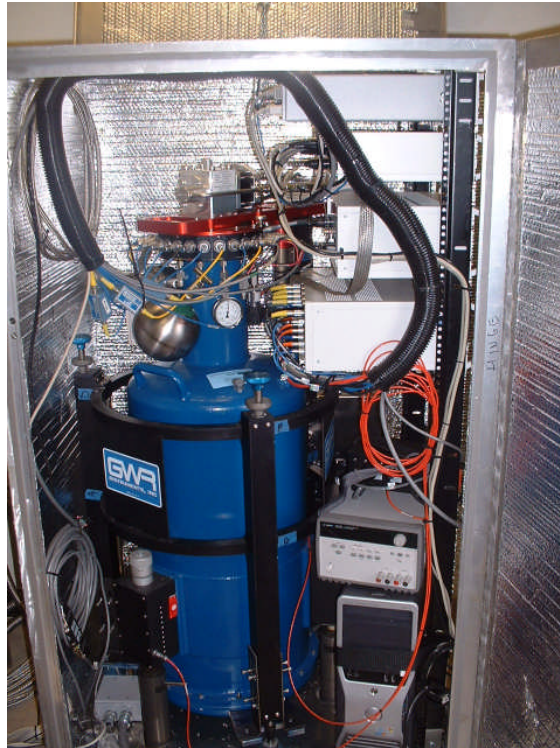
Figure 5: The gravimeter enclosure contains a standard SG, with rack mounted instruments. Transport requires locking the gravimeter dewar to the frame with brackets, and lifting off the gravimeter pillars. Relocations is accomplished with the proof mass suspended.
