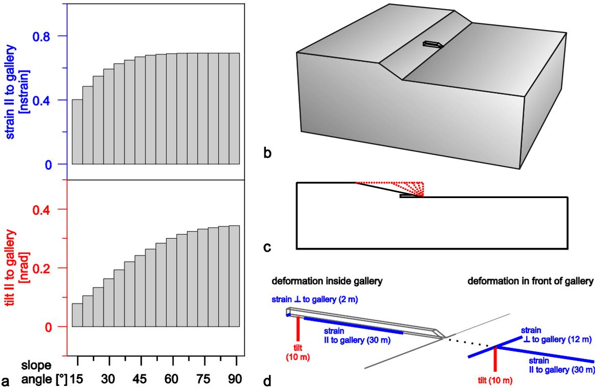
Fig. 1: Determined deformation (a) for a slope model (b) related to a changing slope angle (c). The deformation additionally is determined in front of the gallery (d) as reference.
