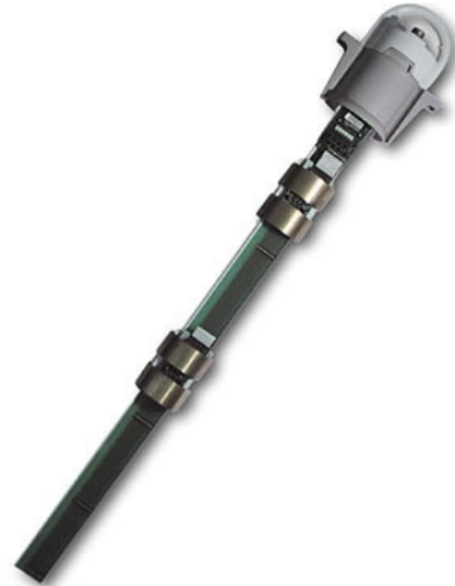
Figure 4: C-Probe used for soil moisture measurement.
