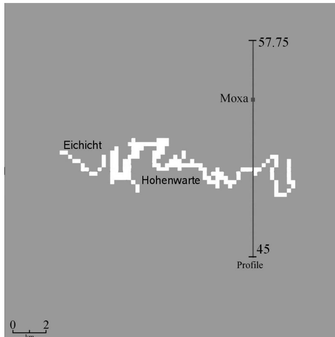
Figure 2: Top view of the model center (20 km x 20 km) with the shape of the reservoirs (white) and the profile for the deformations. The location of the observatory is marked. Numbers indicate locations in km relative to the entire grid of 100×100 km used.
