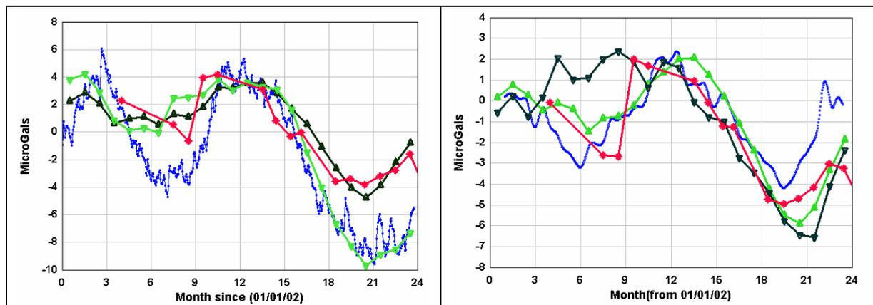
**Figure 3.** Direct observations of gravity field variations from two superconducting gravimeters located in Wettzell (Germany) and in Medicina (Italy). The SG gravity observations are shown in blue and the GRACE observations are shown in red. Predicted gravity changes from the GLDAS output are shown in green (triangles up) (raw, unsmoothed) and black (triangles down) (spatially smoothed to mimic GRACE observations) (from Andersen et al. 2005b).
