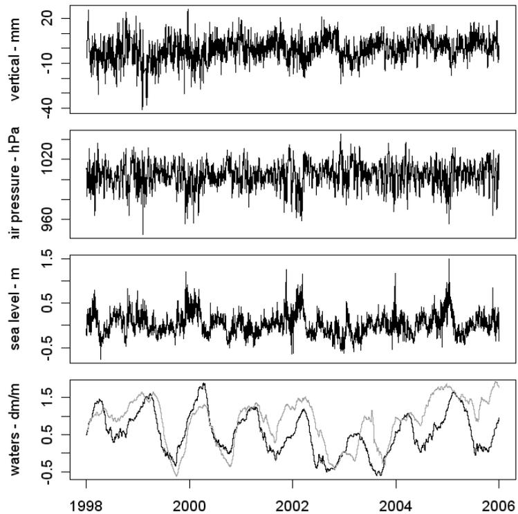
**Figure 3.** The time series data 01/1998 – 12/2005. On top the GPS height (standard deviation 7.4 mm) of Metsähovi corrected for land uplift, second from top is the local atmospheric pressure, second from bottom the sea level time series of Helsinki tide gauge and at the bottom the total water storage of Finland (black, in dm) and local groundwater in Metsähovi (grey, in m).
