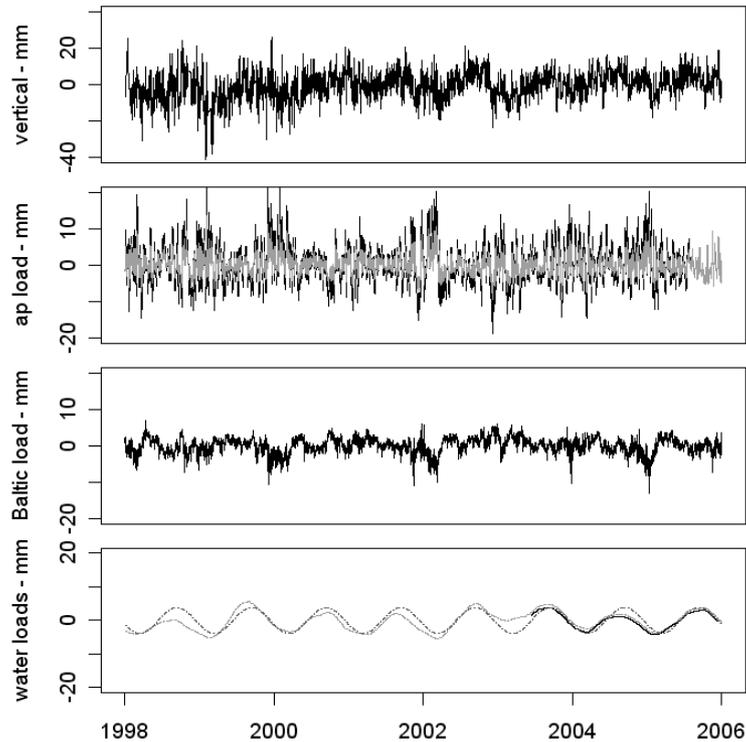
**Figure 4.** The calculated loadings for the different factor 1998 – 2005. On top the GPS time series, second from top the atmospheric pressure loads from HIRLAM (black) and using coefficient (grey), second from bottom the load caused by Baltic Sea and on bottom the calculated watershed loads (CPC model on grey, mixed model on black, starting 06/2003) and a sine function (grey, dashed line). All the loading factors have the same scale (40 mm).
