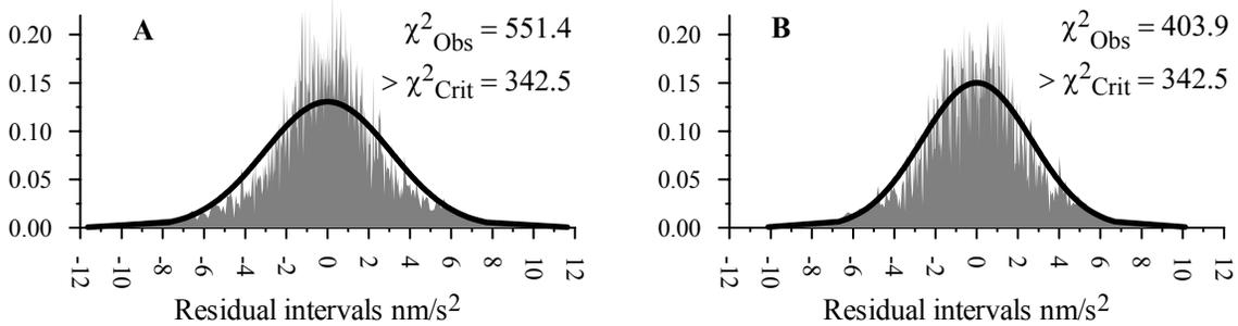
Figure 6. Observed density distribution of the residuals at  $f = 1$  cpd (filed grey curve) and the corresponding ND (thick line). A: all residuals; B: eliminated large residuals (7.5% data).
