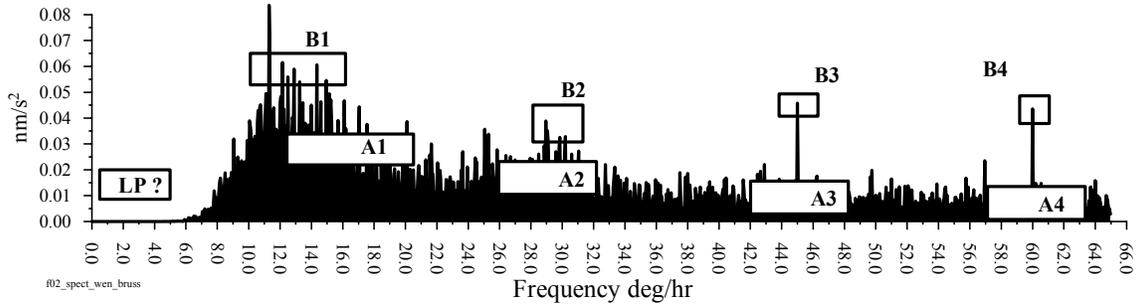
Figure 1. SG data Brussels, ETERNA spectrum of the residuals, obtained with application of the Pertsev filter. The average noise levels  $L(f)$  at the frequencies  $f = 1, 2, 3$  &  $4$  cpd (cycles/day) are determined as arithmetic means of the amplitudes in the intervals, given in Table 1 and indicated in Figure 1 by A1, A2, A3 & A4 respectively.
