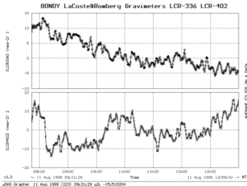
Fig.6: Gravity changes from 9:21 to 13:00 on August 11, 1999 at Bondy station. The two curves show the de-tided records of gravity changes for the gravimeters LaCoste&Romberg 336 (top) and LaCoste&Romberg 402 (bottom). The first and last contacts at Bondy station are about 9:00 and 12:00 respectively, with totality at 10:30.
