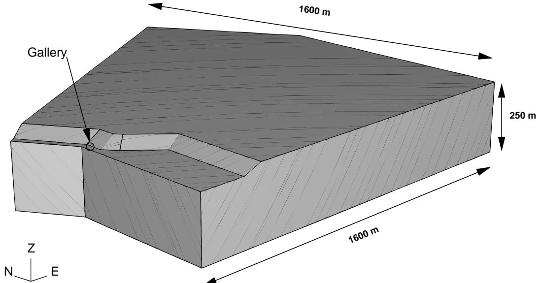
Figure 1: The FEM-model of the Geodynamic Station Moxa and its vicinity. The location of the gallery entrance is marked with a circle. Only the eastern part of the valley is included in the model.
