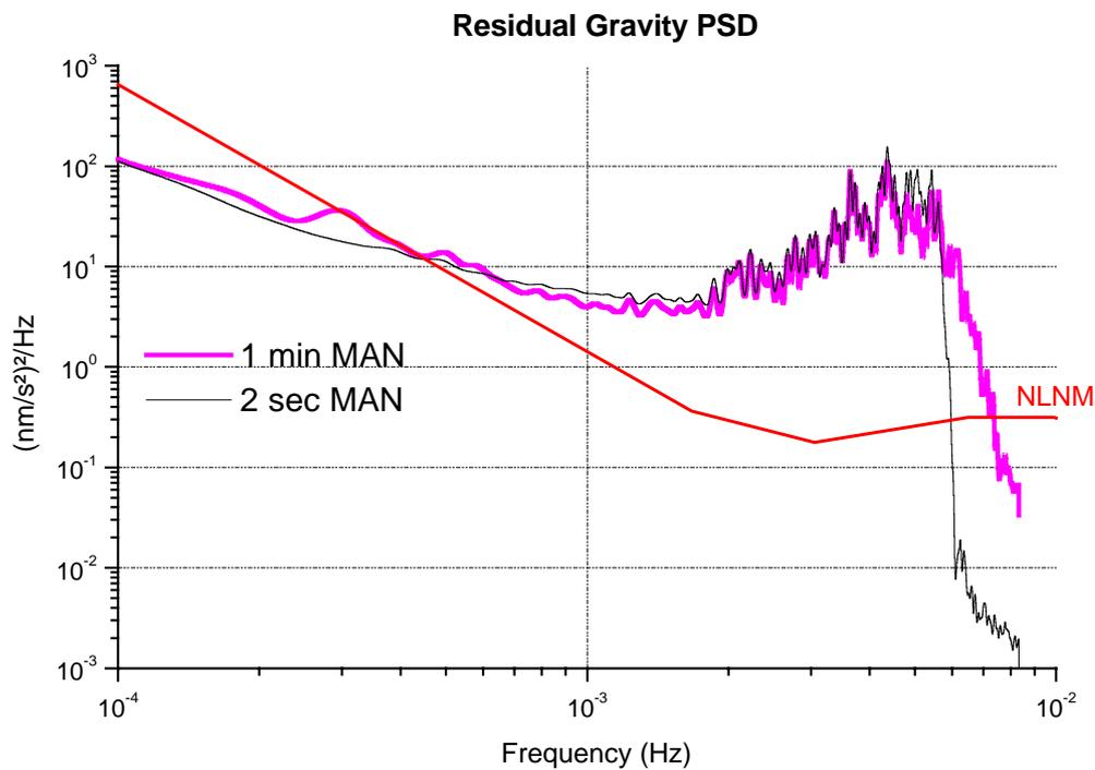
**Figure 10.** Residual gravity PSD according to manual corrections either on raw 2 sec data (further decimated using TSOFT filter) or on 1 min data.
