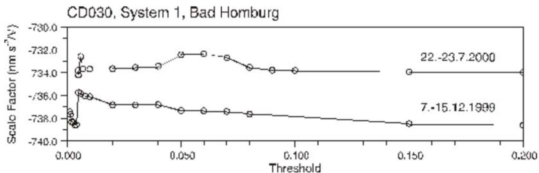
**Fig. 4:** Dependence of the scale factor on the applied threshold of the skew test. The threshold is lowered until the number of detected outliers exceeds about the half of the original number of AG data
