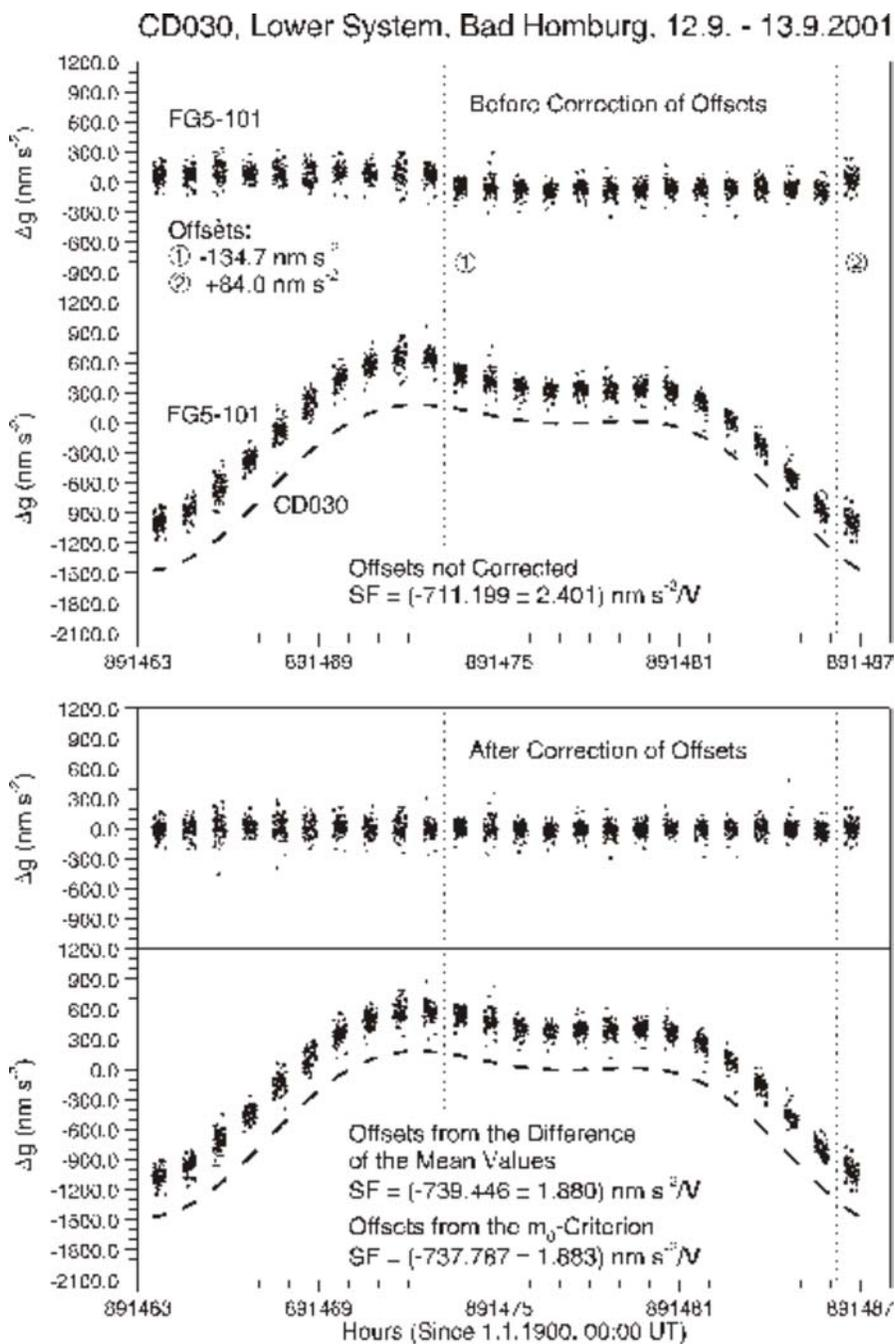
**Fig. 2:** Tidal signals measured by AG and SG. AG data influenced by offsets (Example of the CD030, Bad Homburg, 12.-13.9.2001)
