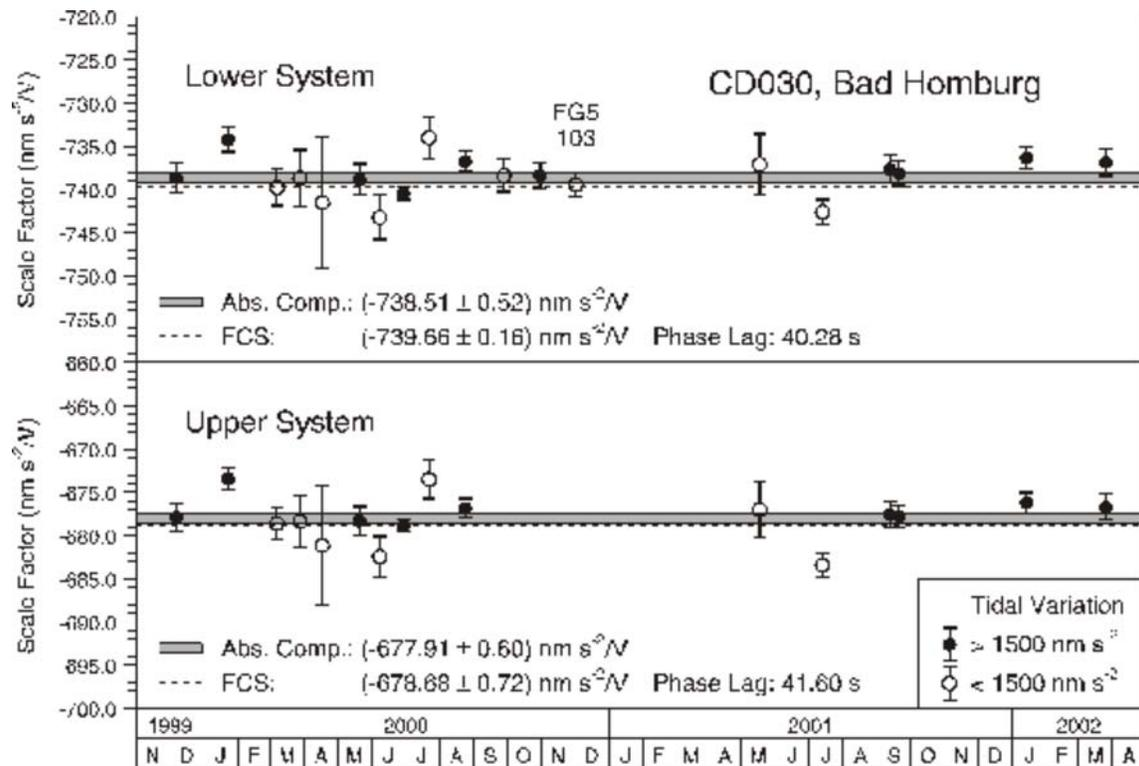
**Fig. 7:** Scale factors of the CD030, derived by comparisons with AG. Grey stripe:  $\pm 1\sigma$ -range of the weighted mean of the 19 single values (The strongly deviating result of calibration no. 19 was not included). Broken lines: results of the Frankfurt Calibration System (FCS), state of March 2002
