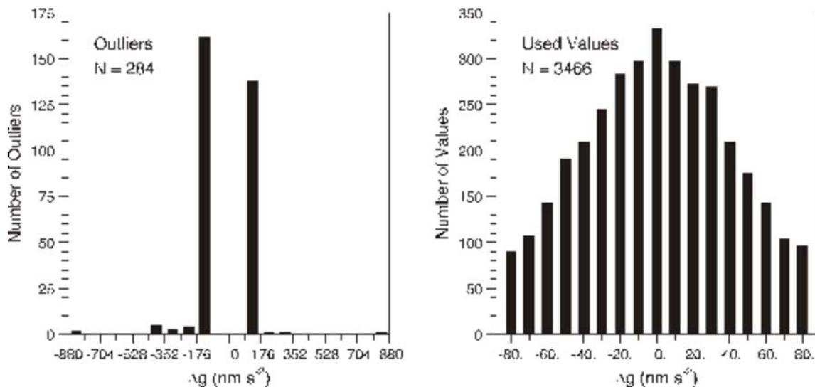
**Fig. 3:** Frequency distribution of the single drop values during a measuring campaign with the AG (Example FG5-103, Bad Homburg, 2.-3.12.2000). On the right: central part of the histogram. On the left: tails on both sides of the histogram, showing the skew of the frequency distribution
