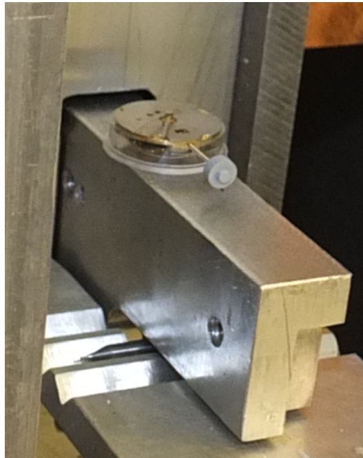
Figure 6: Example of a solar watch mounted on a pendulum pivot for testing
