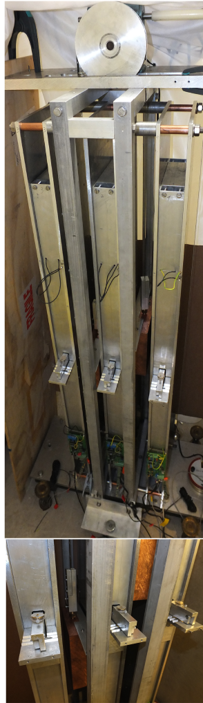
Figure 10: Picture of the set of 3 pendulums (each equipped with a calibrated watch), with a couple of attractive masses, moving vertically up and down. The gravitational torque on each pendulum is directly measured by comparison with two torques of the watches needles.
